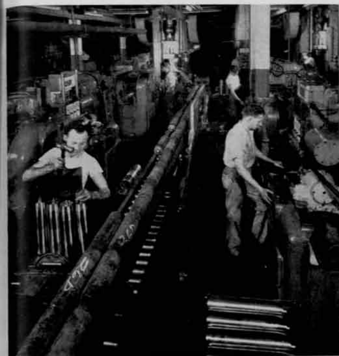
Shellmaking is an intricate process. Cases shown are being rough turned.
