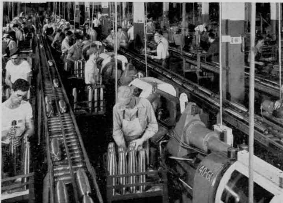
Here shell noses are being threaded. This machining operation must be fast, accurate.
