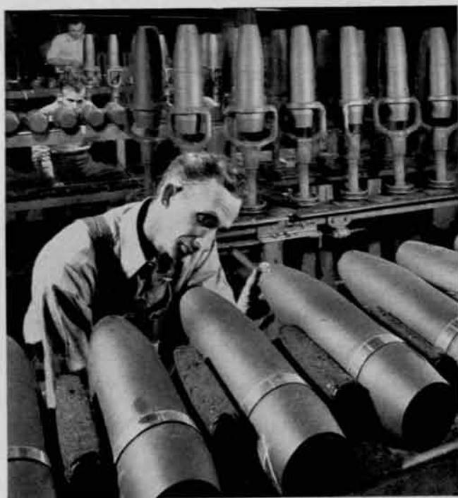
Shells undergo many inspections. Here cases are being checked with a light.
